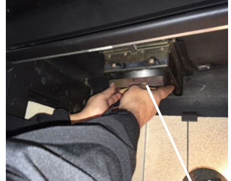
Install square support and catalyst into cartridge
