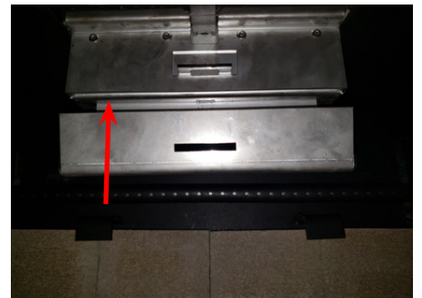
Install square support and catalyst into cartridge
