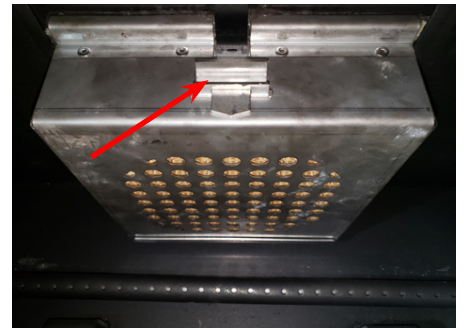
Install flame shield into rear flange and reinstall locking clip removed in Step 1
