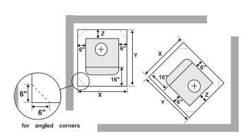
NOTE: In Canada, floor protection must extend 18" to the front and 8" to each side of the stove.
