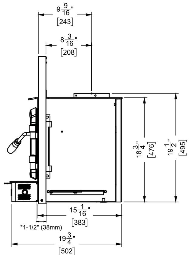
\*Measurement from back of faceplate to fuel door opening
